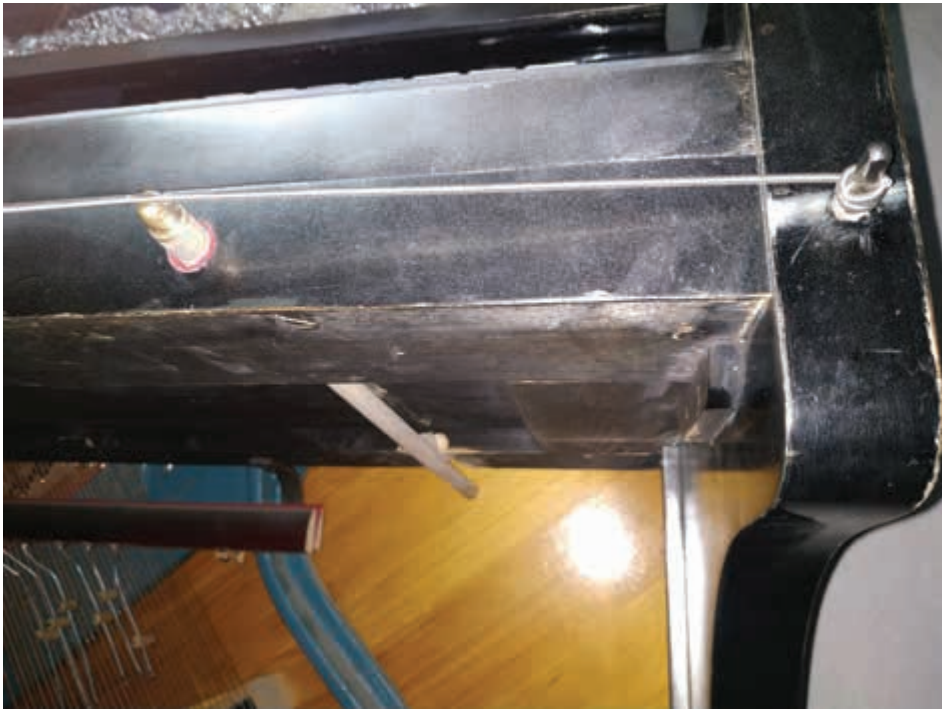
Figure 2: The wooden stick connecting the harp string to the resonator board
